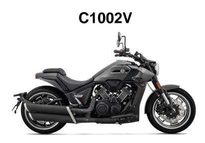
ENGINE V-twin DISPLACEMENT 997 cc **RATED OUTPUT** 70.0 KW at 7600 r/min MAX. TORQUE 102.0 N-m/6500 r/min **COOLING SYSTEM** Liquid-cooled LENGTH / WIDTH / HEIGHT 2380mm / 918mm / 1120mm SEAT HEIGHT 680 **GEARBOX** 6 Speed TANK CAPACITY 22L
